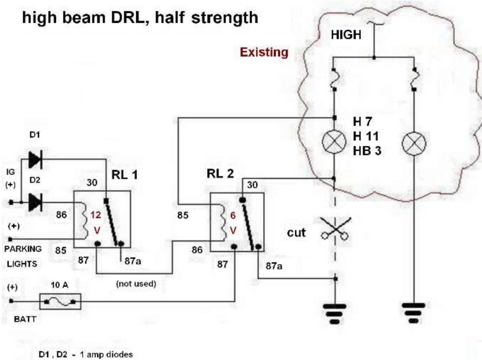
Fig.14. DRL double filament
