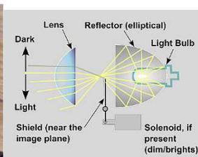
Fig.7. Projector type headlight geometry
