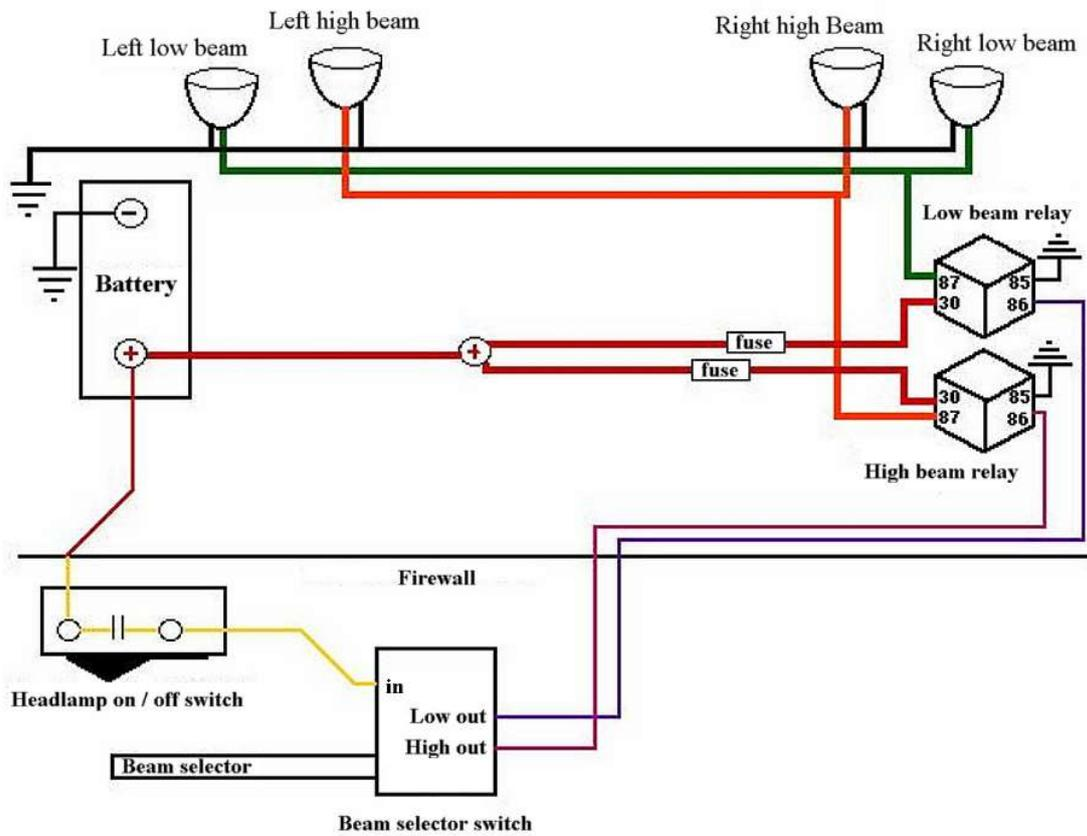
Fig.10. Lighting system with single filament bulb diagram
