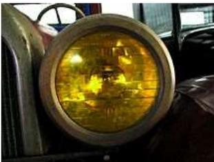
Fig.1. Acetylene headlight
