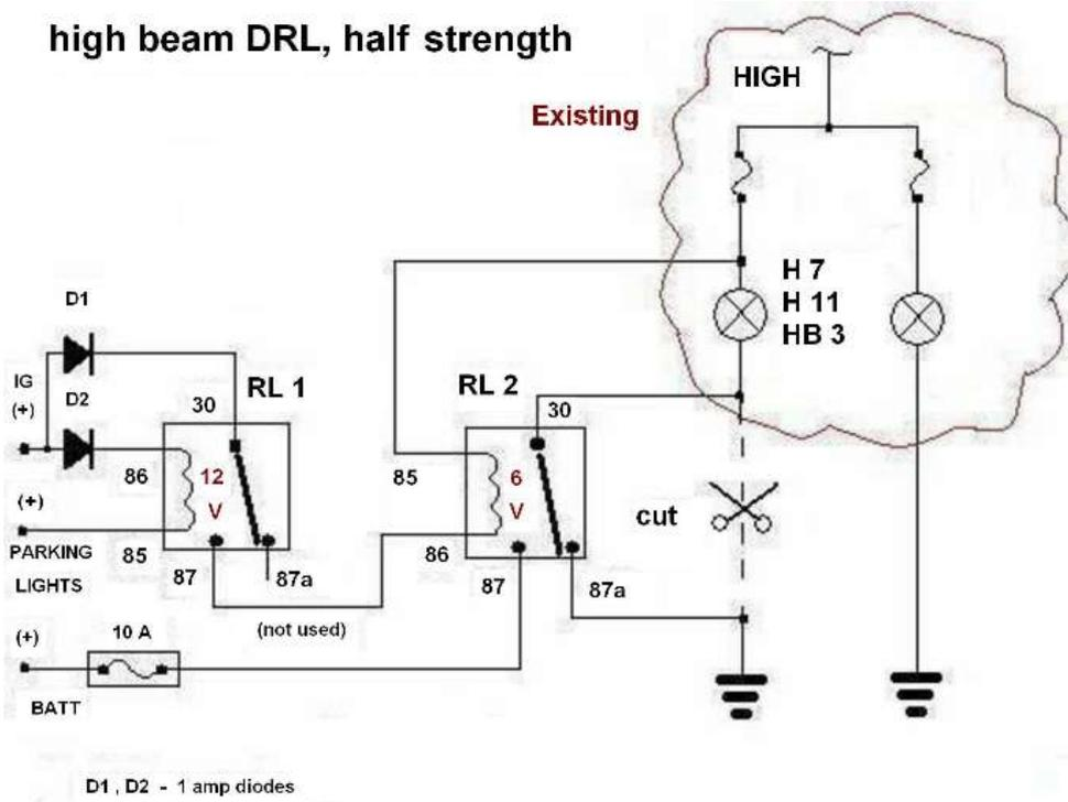
Fig.14. DRL double filament
