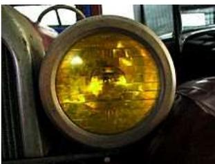
Fig.1. Acetylene headlight
