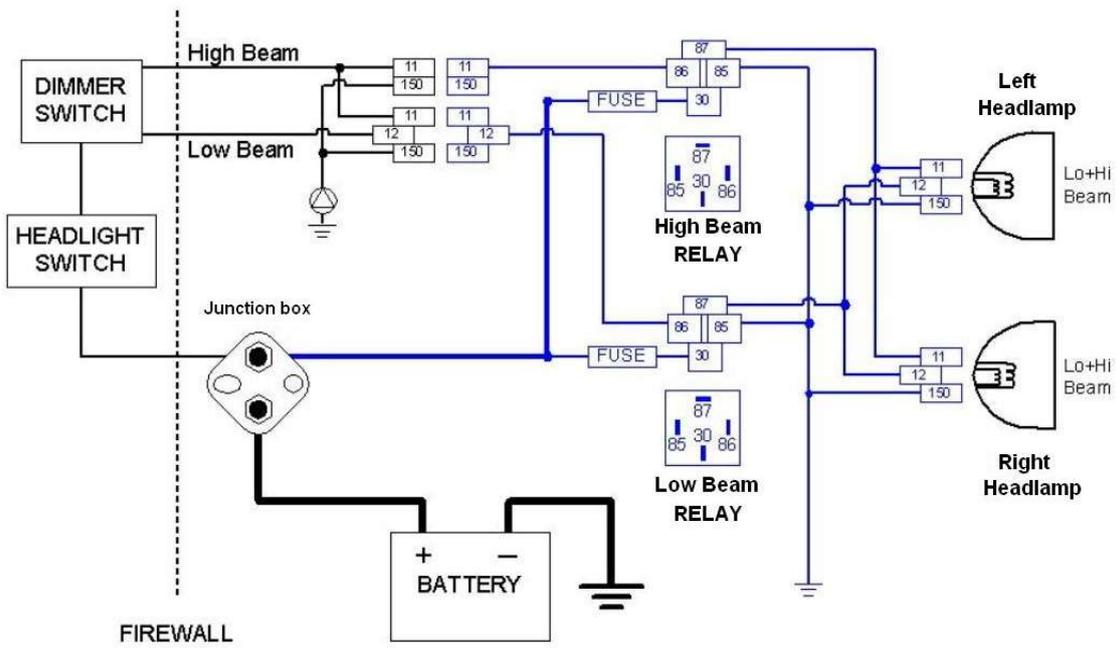
Fig.9. Lighting system with double filament bulb diagram
