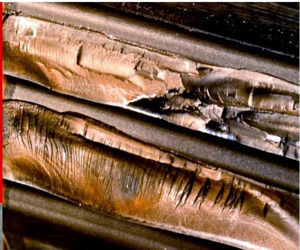
4 Bending Fatigue/High-Cycle/Root Fillet Cracks
