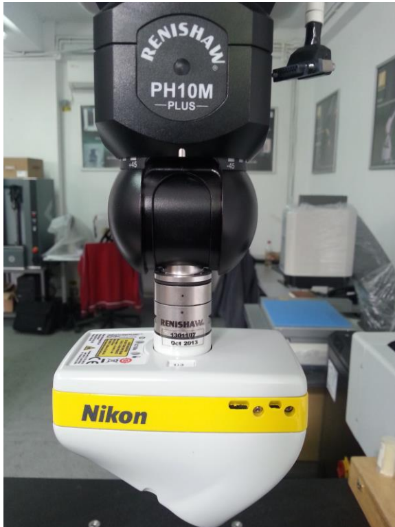
Fig. 24 Laser NIKON LC15Dx
